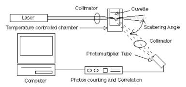
**Diagram 1.** Illustrates the workings of the experiment which employs a dynamic light scattering system of the type Malvern.
